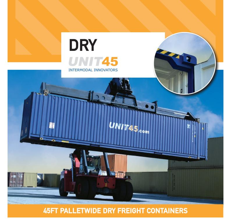
UNIT45's 9ft 6in high palletwide dry freight container offers the highest cubic capacity and payload of any standard 45ft container design. By using special high-strength steels and lightweight floor materials,
