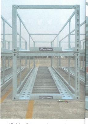
(in this case even up to eight pieces) with the use of standard container handling equipment. By fewer vehicle handlings and lashings, damages can be reduced. Lastly in this regard, VUCAFrames can increase terminals and compounds' storage space by a factor of three, as the frames can simply be put one onto another, something which cannot be done with "bare" cars. What's important, too, the VUCAFrame
