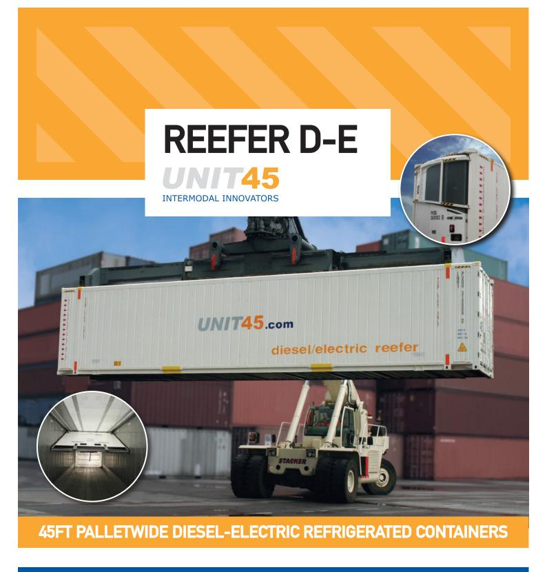
UNIT45 has developed a diesel-electric reefer container primarily intended for use in multimodal operations where rail is featured. The cost of moving temperature-controlled cargoes over long distances by road is ever rising but rail is rarely an alternative since very few train operators can provide a reliable power supply for all-electric reefer containers.
