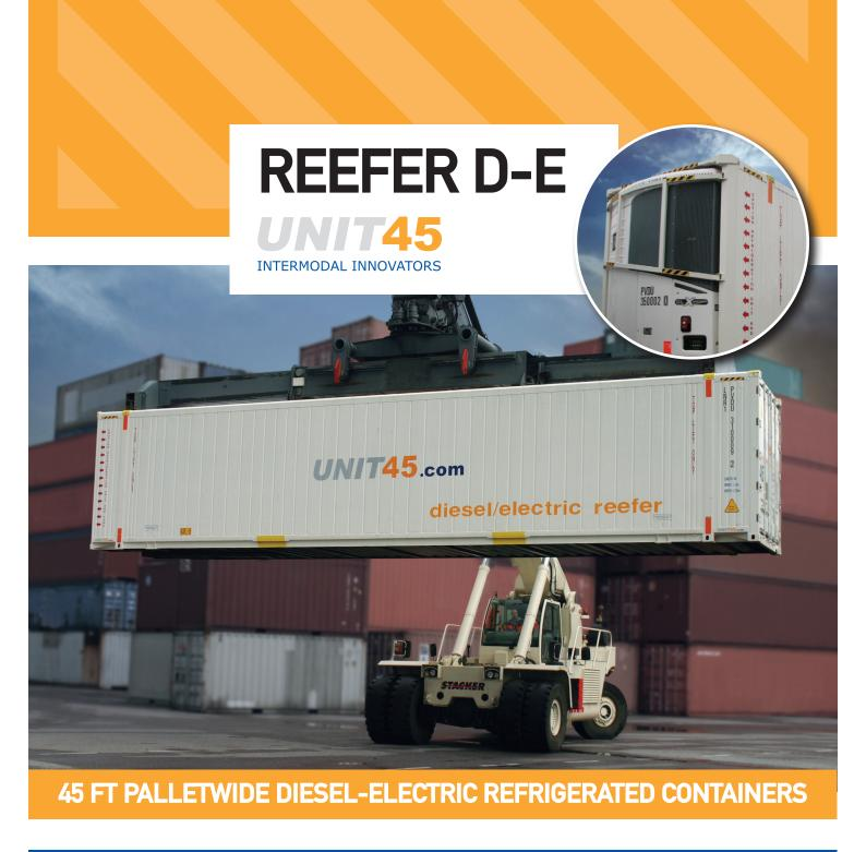
UNIT45 has recently developed a new dieselelectric reefer container primarily intended for use in multimodal operations where rail is featured. The cost of moving temperaturecontrolled cargoes over long distances by road is ever rising but rail is rarely an alternative since very few train operators can provide a reliable power supply for all-electric reefer containers.
